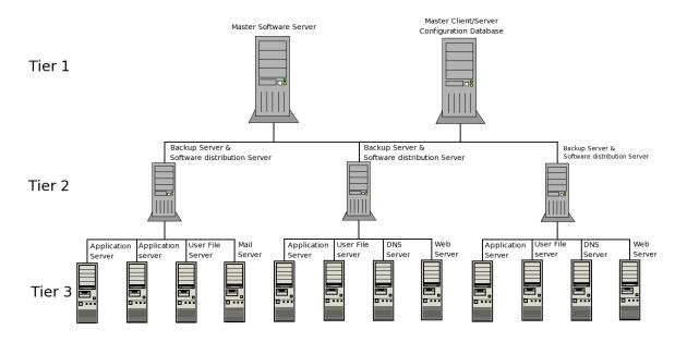
It should be noted that the differences in functional behavior of the servers in tier 2 and 3 of this diagram are not based on there being differences in the software but rather as a result of differences in the configuration files that enable and disable the functionality of a particular server.
